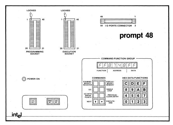
also provides 1K of writeable program memory which may be used to debug user programs. A multiple single step feature is also provided in which the processor steps through its program dumping all internal contents to external RAM where it may be later displayed or typed out on an external terminal. Paper tape input and output in Intel's hexadecimal format is also available through the TTY.
